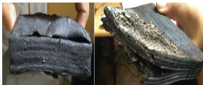
Coated v/s bare wood specimen at 400°C
