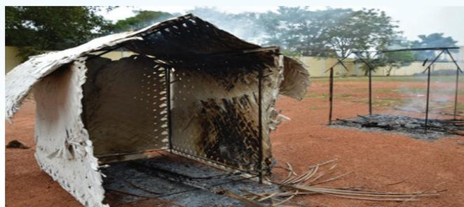
*Fig. 1 Model huts made of thatched coconut leaves set to fire. (Left)-Hut without CASPOL coating gutted completely in fire within a few seconds whereas CASPOL coated hut remained intact even in fire.*
