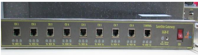
Front panel of 9-channel SGU
