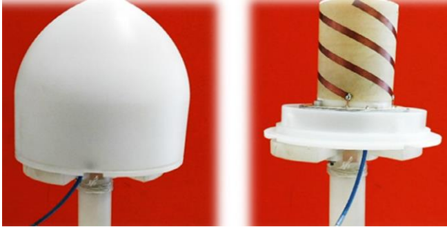
Tx Antenna for Pole
