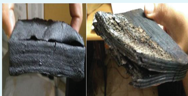
Coated v/s bare wood specimen at 400°C
