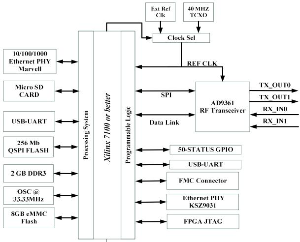
BLOCK DIAGRAM FPGA BASED SDR HARDWARE
